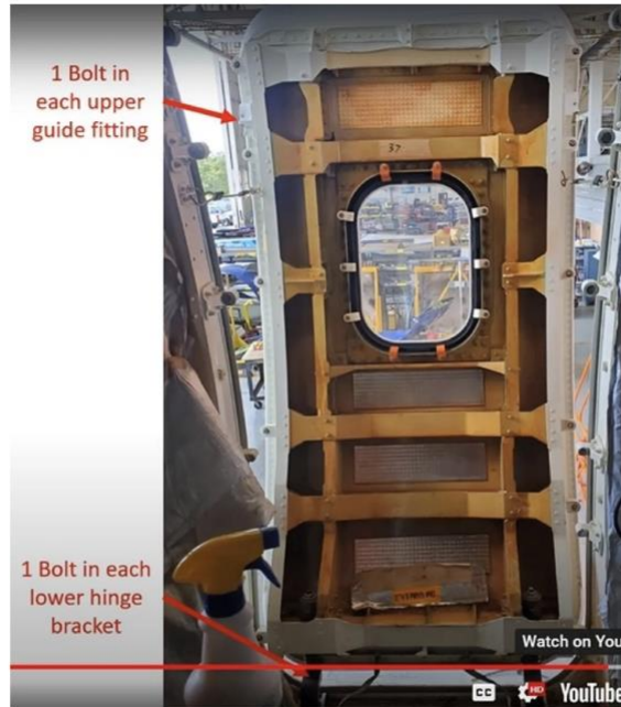
A photo showing the type of door plug fitted to a Boeing MAX 9 aircraft that fell off Alaska Airlines flight 1282. It's secured to the airframe by two bolts at the top and two at the bottom. (Courtesy of Chris Brady at b737.org.uk)
